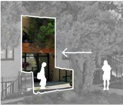
4.5.3 Recess entryways for weather protection
