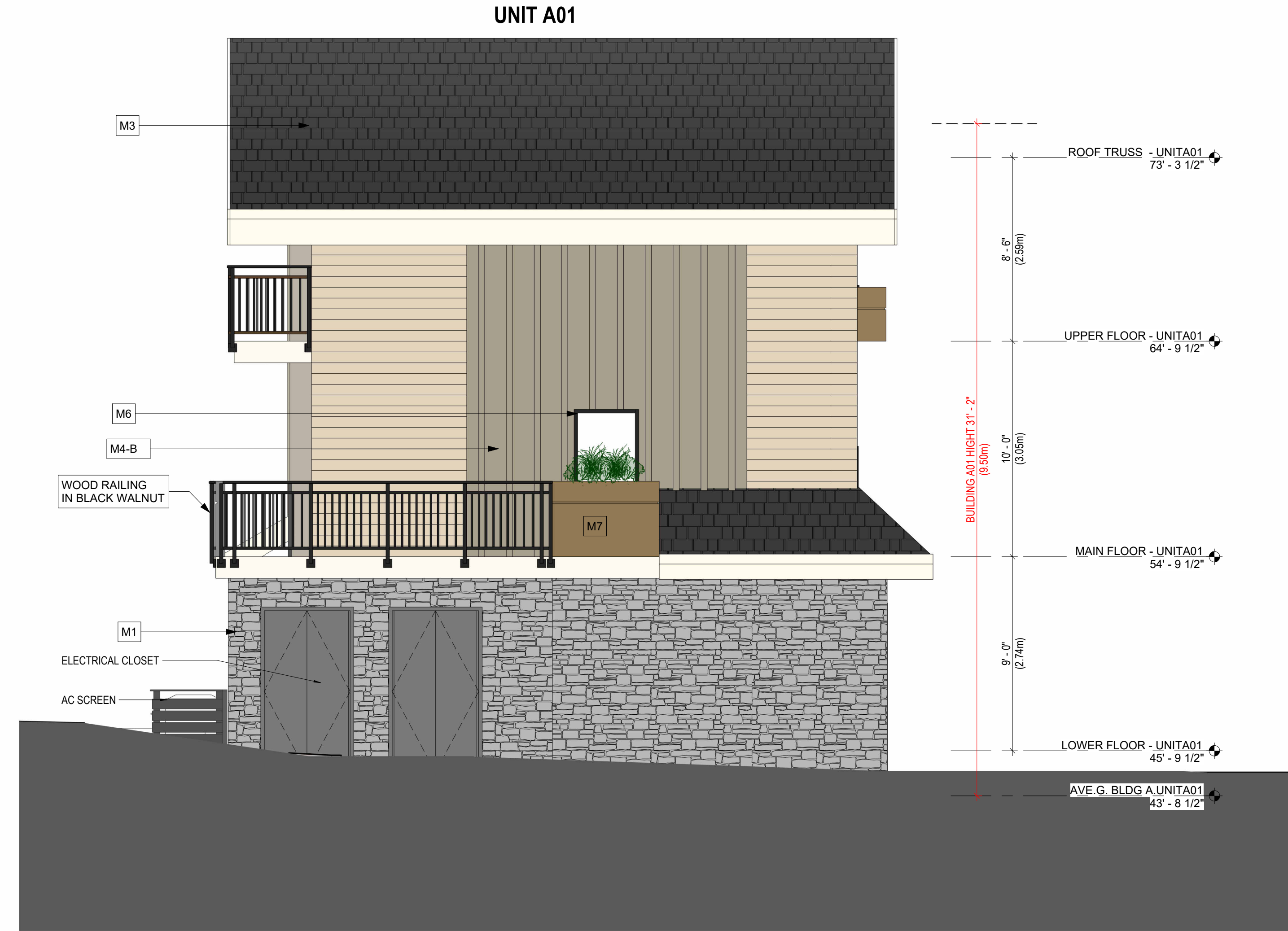
2 BUILDING A - SOUTH ELEVATION SCALE: 1/4" = 1'-0"
