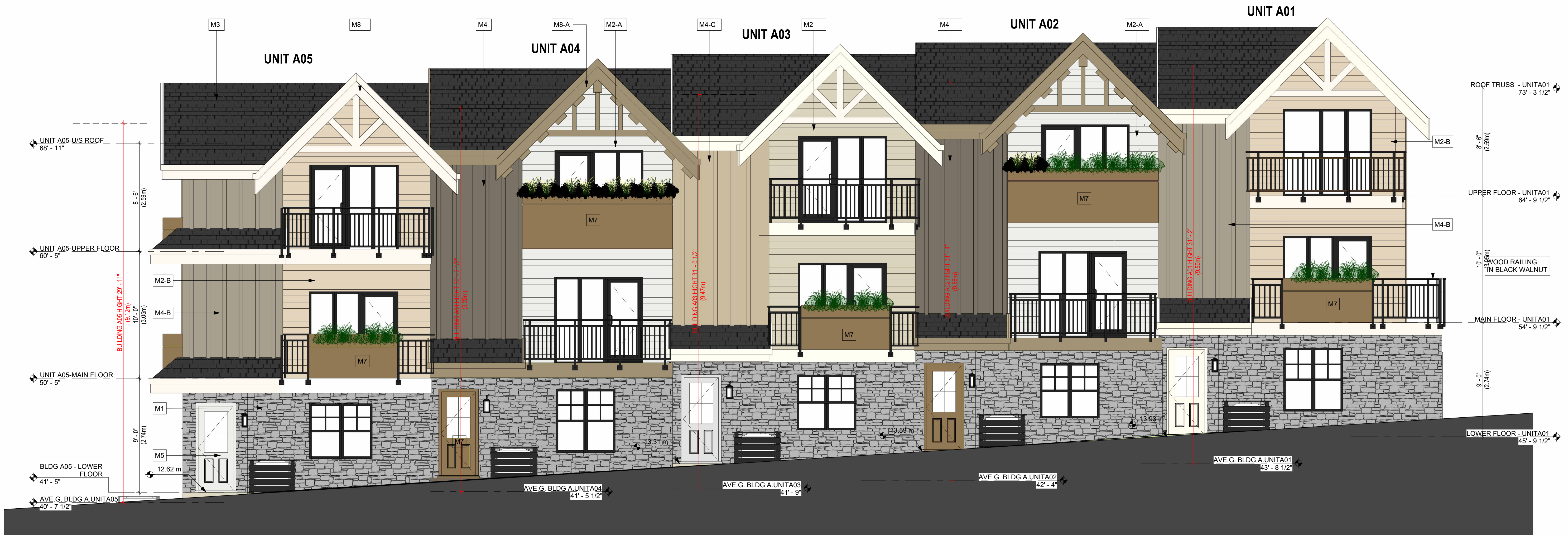
1 BUILDING A - WEST ELEVATION SCALE: 1/4" = 1'-0"
