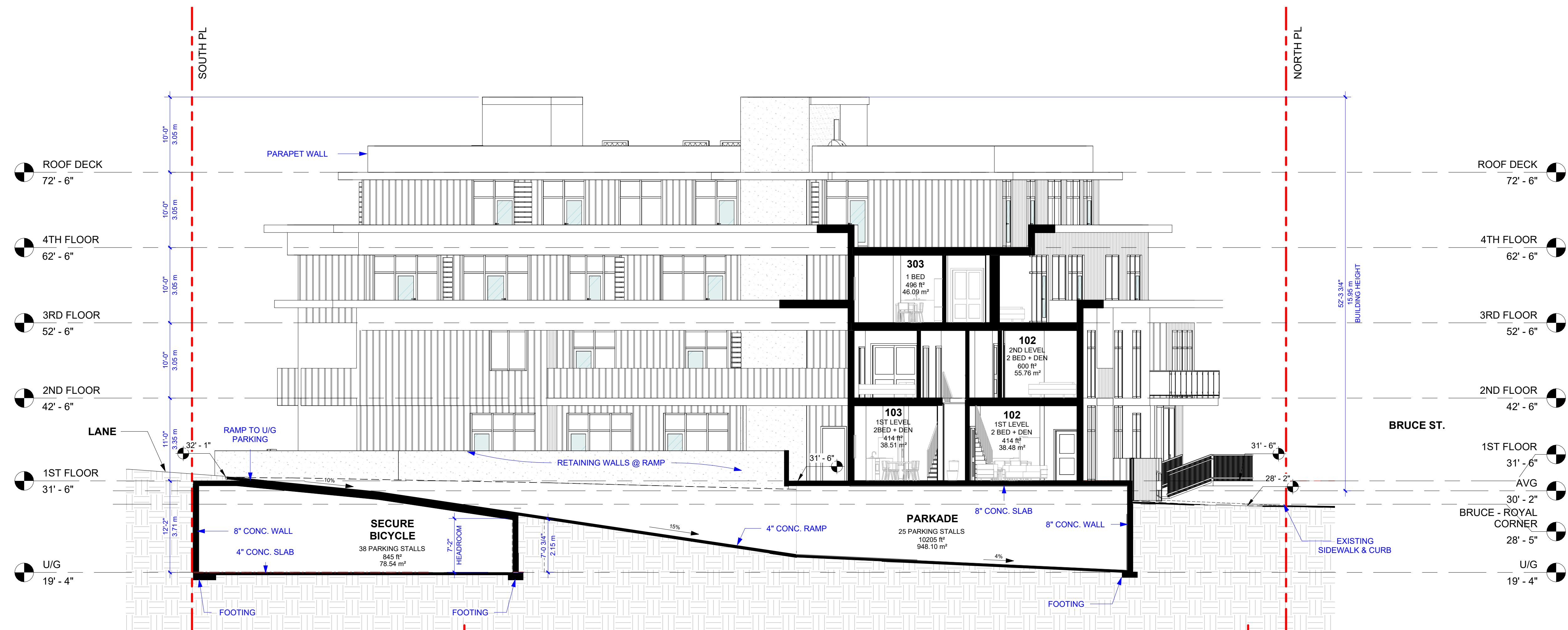
① U/G PARKING RAMP SECTION VIEW 1/8" = 1'-0"
