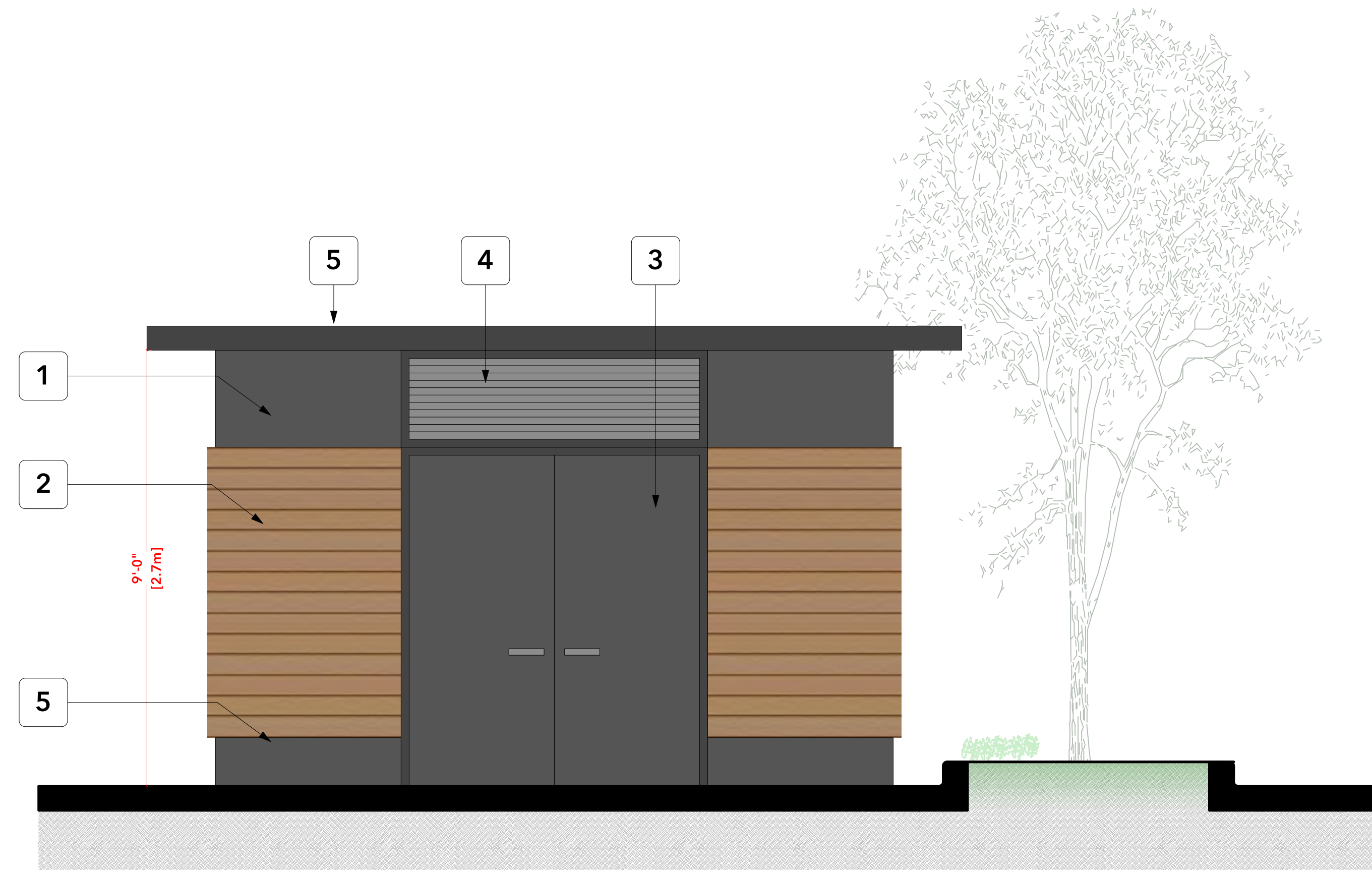
3 SOUTH ELEVATION Scale: 1/2" = 1'-0"
