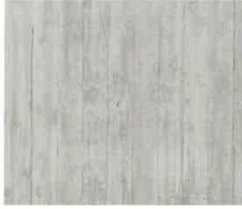
Board Formed Concrete
