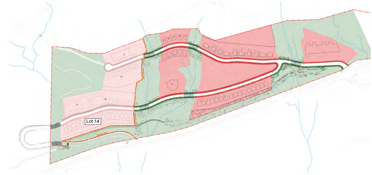
Area 6 Plan - Preserved Forest Management Zones (shaded green) vs. Development Parcels: Phase 1 (shaded dark pink) & Phase 2 (shaded light pink)
