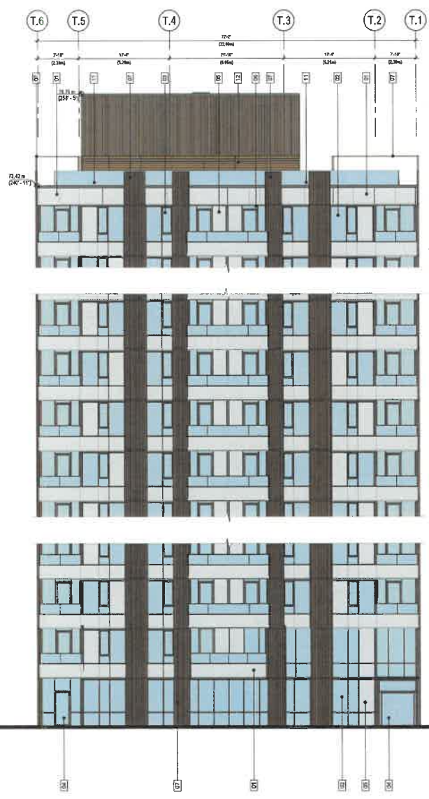
2 ENLARGED BUILDING ELEVATION - NORTH 1/8" = 1'-0"
