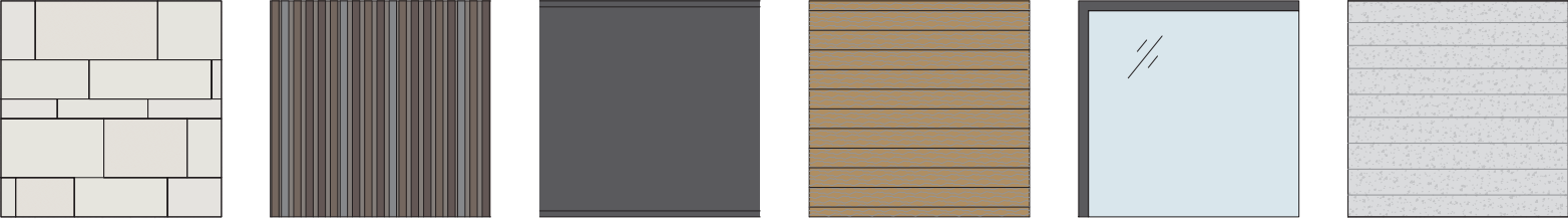
① LIMESTONE WALL CLADDING ② FIBER CEMENT WALL CLADDING ③ METAL ROOF TRIM ④ WOOD SOFFIT ⑤ TRIPLE GLAZED WINDOWS ⑥ BOARD FORM CONCRETE WALL
