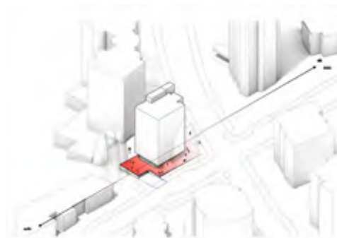
5. Lift massing at ground floor to link the site public realm to public thoroughfare along 22nd Street.
