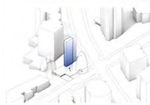
1. Core placement responds to site conditions: parkade entry, adjacent building overlook and tree retention.
