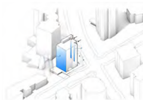
4. Maximizing views to the south with operable windows to the north to provide for cross ventilation through the units.
