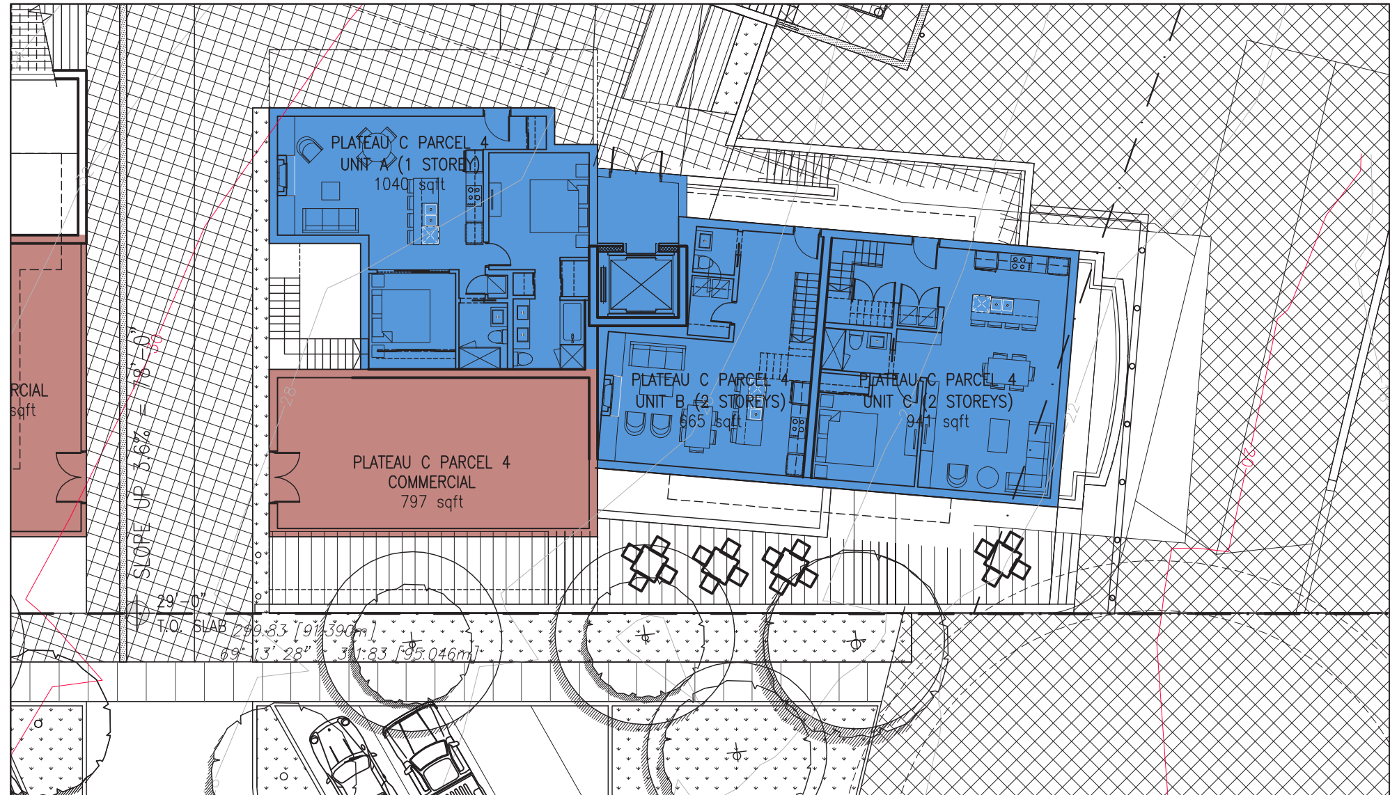
2 Parcel 4 – Level 2 Floor Plan SCALE : 1/16" = 1'-0"
