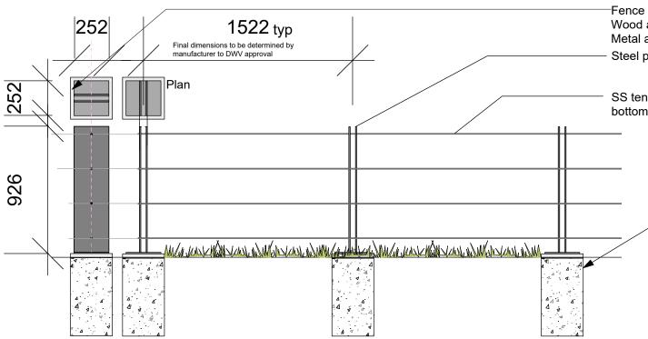
Fence Posts to match existing bollards in size and look-Wood and top plate not required Metal and Cable Gage TBD by contractor & noted in shop drawings - Steel painted post- to match existing lighting bollards
