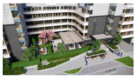
Figure 5 – Rendering of proposal (indicating landscape improvements, elevator glazing, entrance improvements and metal band between brick and cementitious paneling)
