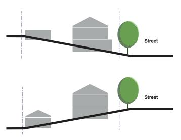
**Fig 2.5:** On both uphill and downhill lots, coach houses need to consider massing implications from the fronting street and the lane, and seek to minimize excavation and exposed foundation walls.
