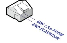
*Fig 3.3:* To manage scale, dormers should be sloped and be set back from the end elevation.
