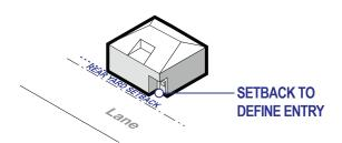
**Fig 3.2:** An entry facing the lane should be set back from the rear property line to allow for safe access.
