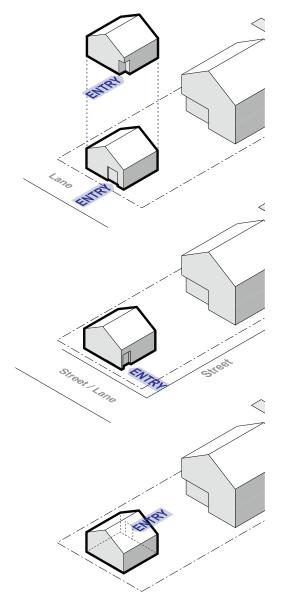
**Fig 3.1:** For lots with a lane or street, the entry should be oriented towards, or be visible from, the lane or street. For lots without a lane, the entry should be located on the side or interior yard.
