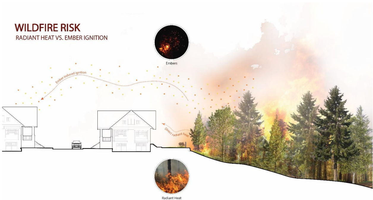
Figure 7. Radiant heat threatens structures within 10m of the forest edge while embers spread to structures within the interior of the development.
