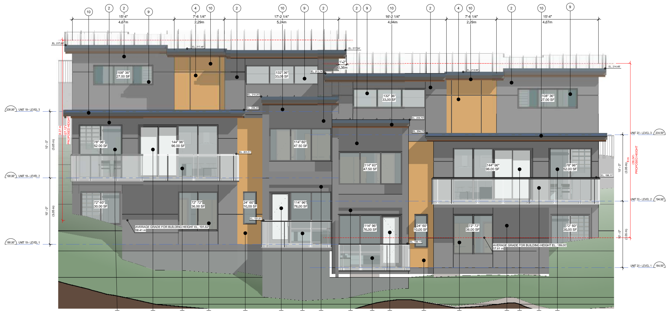
② UNIT 19 & 20 - WEST ELEVATION 1/4" = 1'-0"
