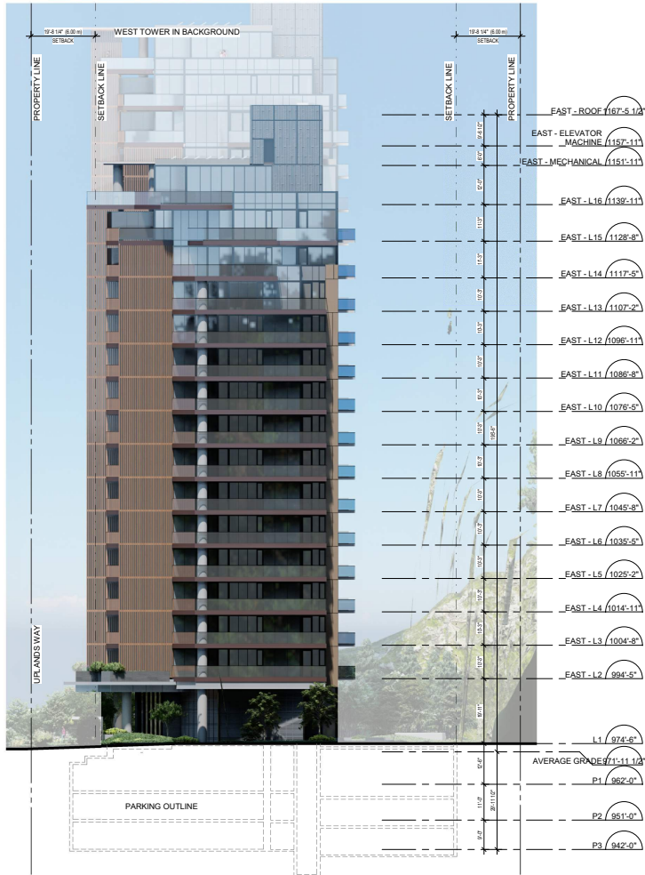
① EAST TOWER - EAST ELEVATION 1/16" = 1'-0"
