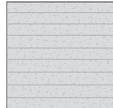
⑥ BOARD FORM CONCRETE WALL
