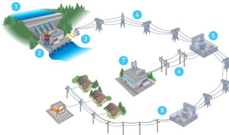
Figure 1. Electricity generation, transmission, and distribution
