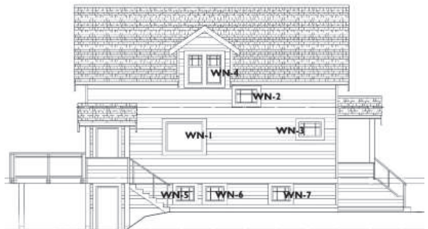
Figure 37: Window Schedule: North elevation
