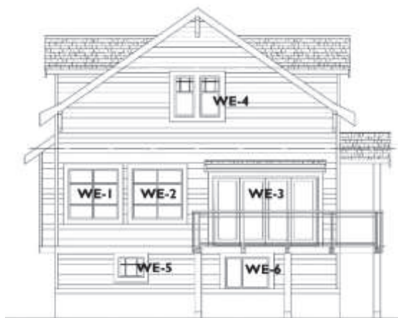
Figure 38: Window Schedule: East elevation
