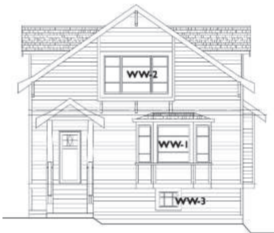
Figure 36: Window Schedule: West elevation
