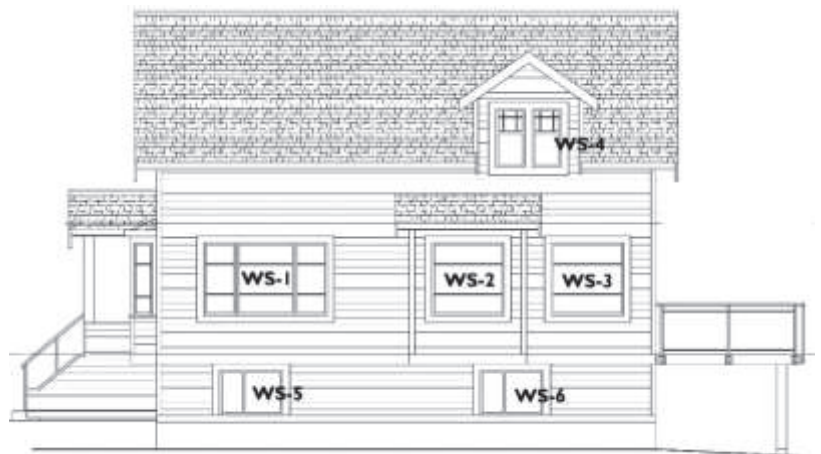
Figure 39: Window Schedule: South elevation
