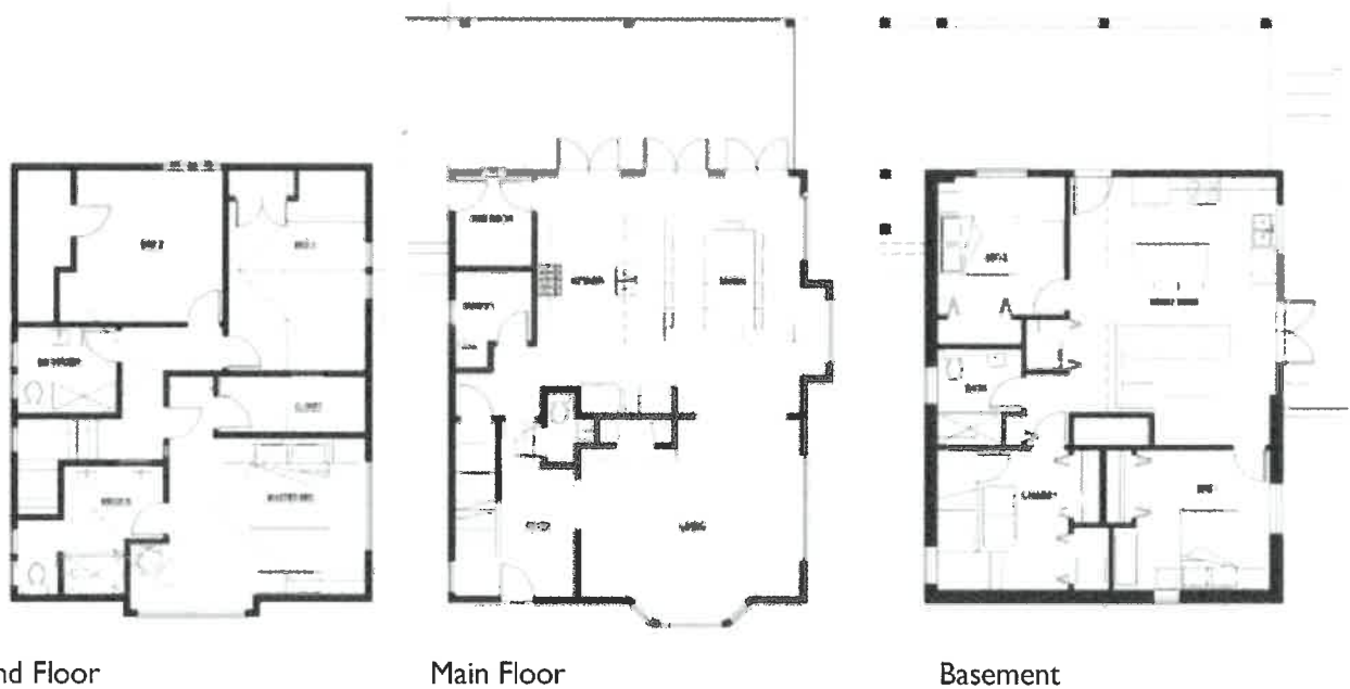
Figure 74: Proposed floor plans with basement suite, main Floor with east facing deck and second floor with added dormers_ Focus Architectural Inc
