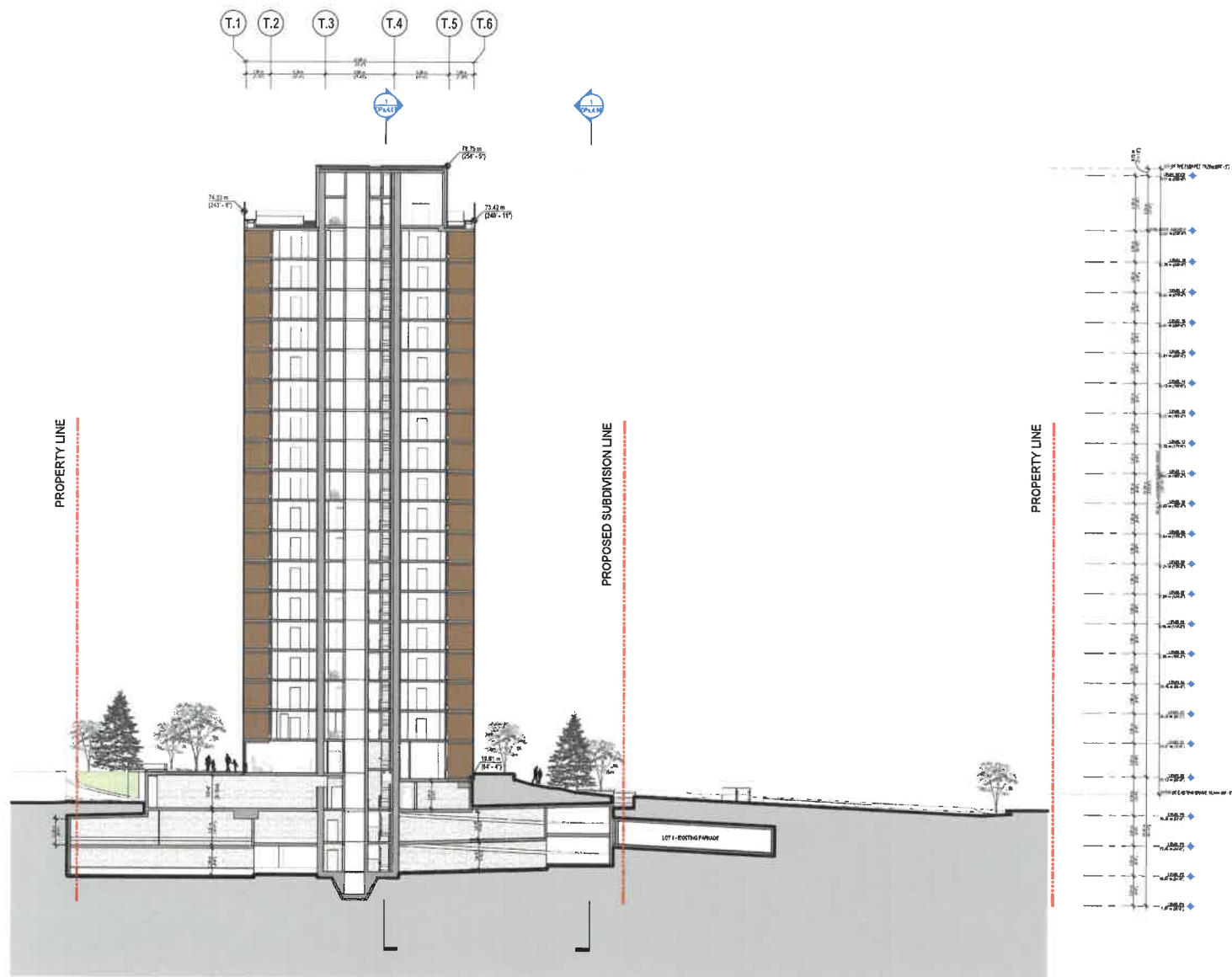
1 OVERALL BUILDING SECTION - EAST-WEST B 1/8" = 1'-0"
