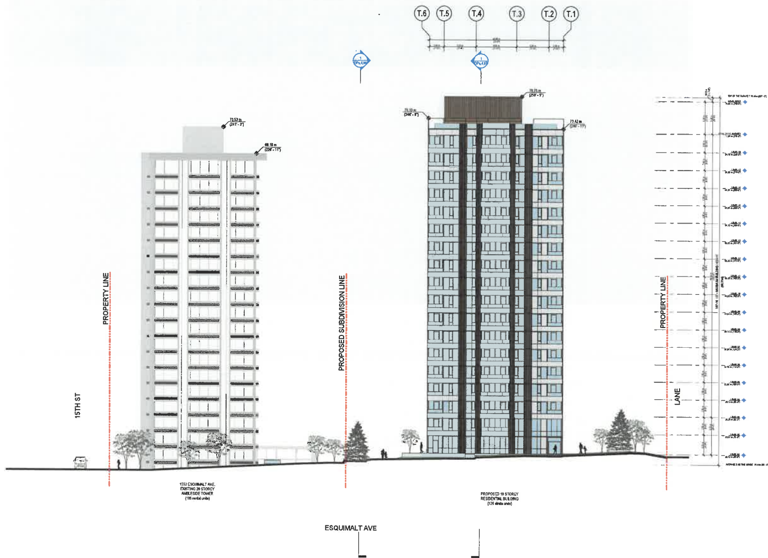
1 OVERALL BUILDING ELEVATION - NORTH 1/16" = 1'-0"
