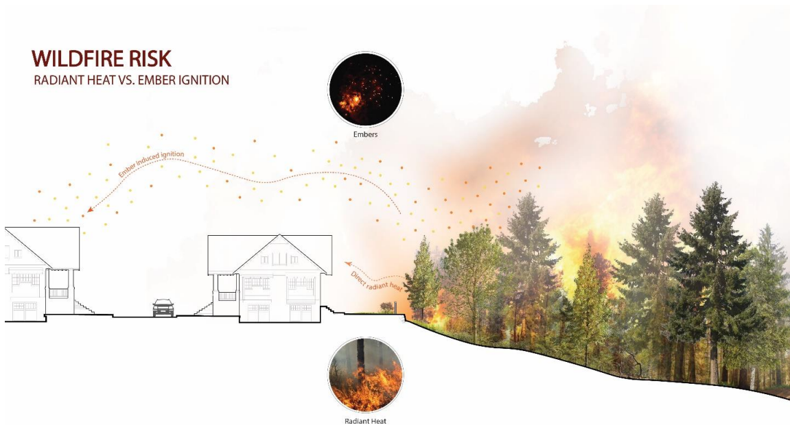
Figure 6. Ignition pathways in the interface. Radiant heat threatens structures within 10m of the forest edge while embers spread to structures within the interior of the development.
