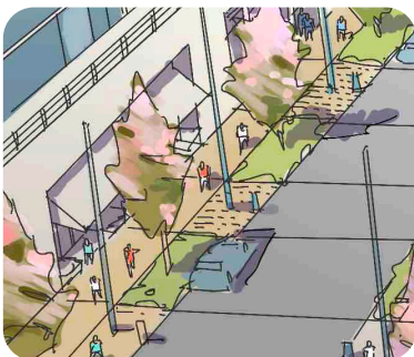
Include purposeful landscaping and make use of permeable surfaces
