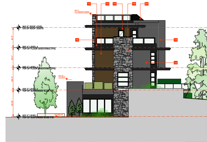
4 Building 1 - South Side Elevation SCALE: 1/8" = 1'-0"
