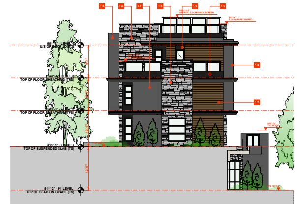
2 Building 3 - North Side Elevation SCALE: 1/8" = 1'-0"
