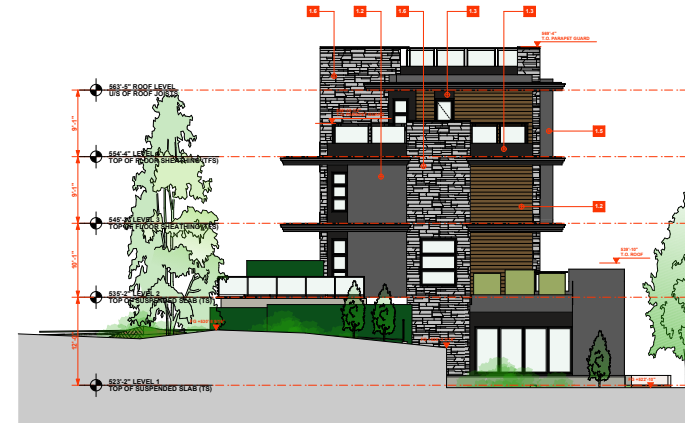
2 Building 1 - North Side Elevation SCALE: 1/8" = 1'-0"
