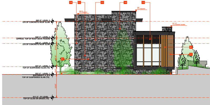
2 Amenity Building - Front Courtyard Elevation SCALE: 1/8" = 1'-0"
