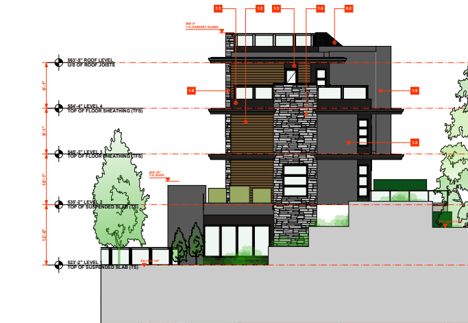
4 Building 2 - South Side Elevation SCALE: 1/8" = 1'-0"
