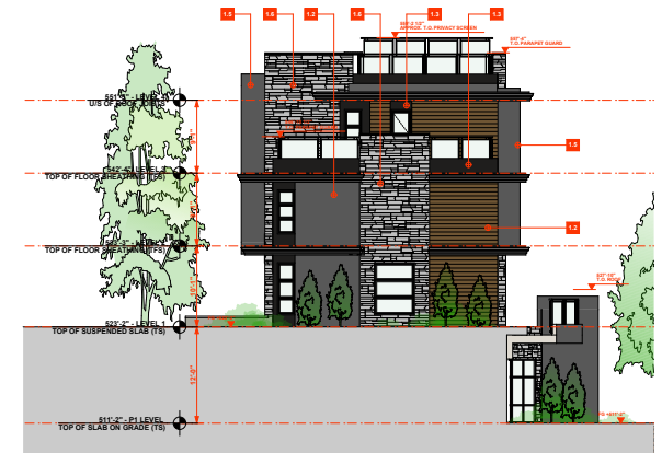
2 Building 3 - North Side Elevation SCALE: 1/8" = 1'-0"
