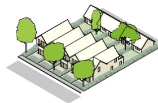
The traditional rowhouse consists of units arranged side by side, each with their own front door and outdoor area.
