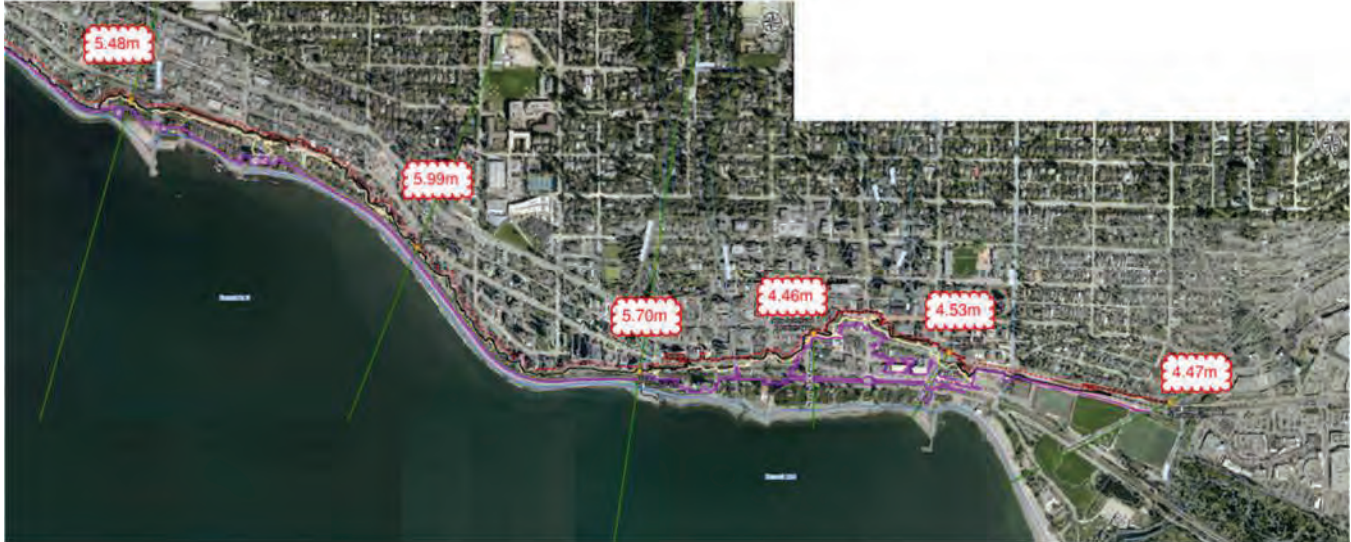
Figure 5.2: Recommended Design Elevations (Elevations shown in red)
