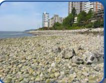
The shoreline at McDonald Creek had historically experiened significant erosion, leaving a low-profile beach vulnerable to continued erosion from waves. Wave erosion can be limited by 'roughening' the shoreline, using large riprap to create an irregular and sloping beach that diffuses wave power before the waves reach the upper shore and Seawalk.
