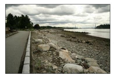
A hard-faced concrete sea wall fronted the centennial Seawalk along the upper foreshore between Lawson Creek and McDonald Creek. The low profile cobble beach offered little natural resistance to waves and wave erosion posed a threat to the shoreline and structural integrity of the sea wall. The low profile beach and sea walk restricted access to the beach to two points. Small pockets of dune grass and salt marsh grew on isolated patches of upper shore with little room for available expansion.
